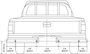
Near the ends of the bumper, mark the same sensor height on masking tape creating 3 points along the bumper. Run a strip of tape so the top of the tape connects all 3 points. (These points will form the drill line), mark with additional strips of tape. To protect the rear corner of the vehicle, mount sensors within 1' from the edge.
